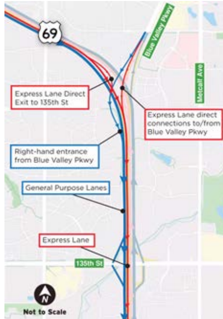
Figure 3 – SB ETL Ramp Configuration
