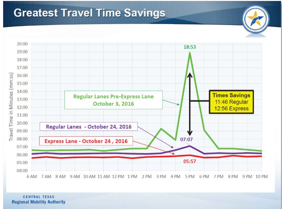
Figure 1 – ETL Travel Time Savings in Austin, TX
