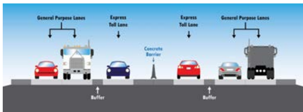
Figure 6: US 69 Express Toll Lane Typical Section
